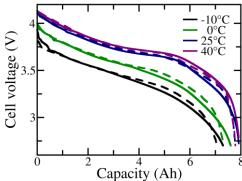
Cell voltage response (measured vs predicted)
