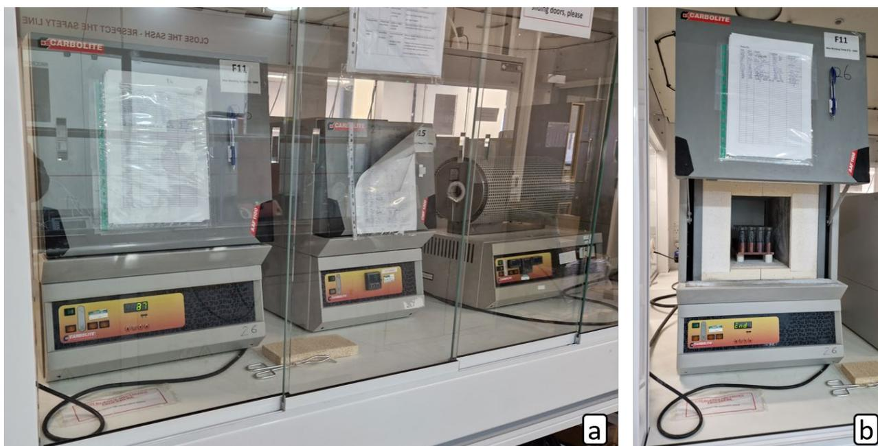
**Figure 6.** Natural convection box furnace placed inside a fumehood (a) in a dedicated furnace lab and (b) the pair of stainless-steel sample racks at the end of a completed calcination step.
