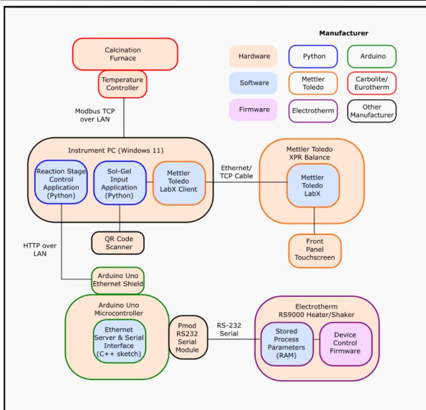
**Figure 7.** Network diagram for software used for the automated process, along with their corresponding hardware components.
