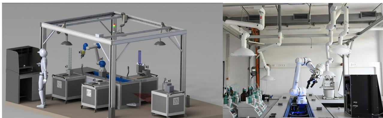
**Figure 14.** Left: Concept illustration of the Fraunhofer ISC setup. Robotic arm (a) installed on a linear axis (f) and equipped with a robotic gripper (g). Liquid-liquid extraction device (c). Magnetic stirrer with heating plate (d). Precision scale / dosing device (e). Rotary evaporator (b). Right: Assembled robot platform.
