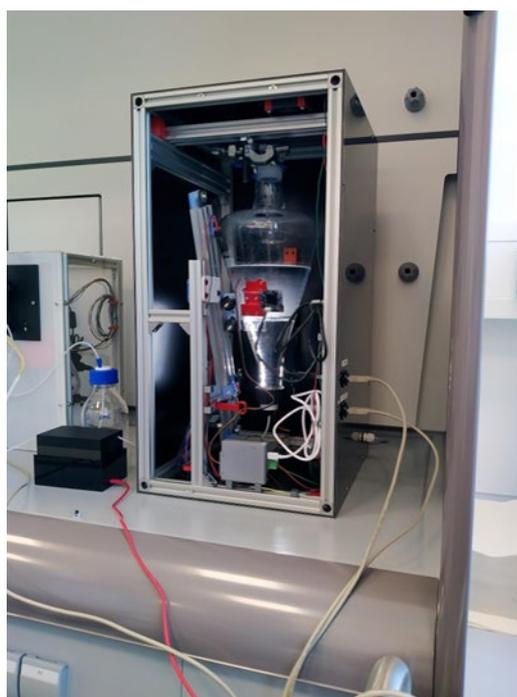
**Figure 19.** LLE module inside a glovebox during a draining step of ethyl acetate and water-polymer solution.
