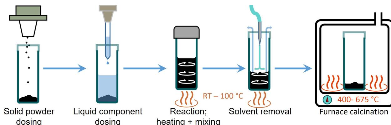
**Figure 1.** The semi-automated coating process of  $\text{LiNi}_{0.6}\text{Mn}_{0.2}\text{Co}_{0.2}\text{O}_2$  (code NMC622) with alumina ( $\text{Al}_2\text{O}_3$ ).
