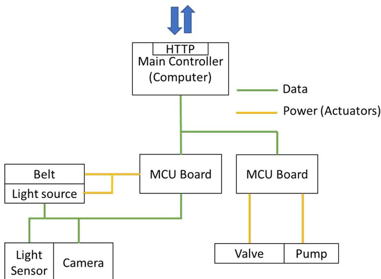
**Figure 16.** Connection and control diagram for LLE device.
