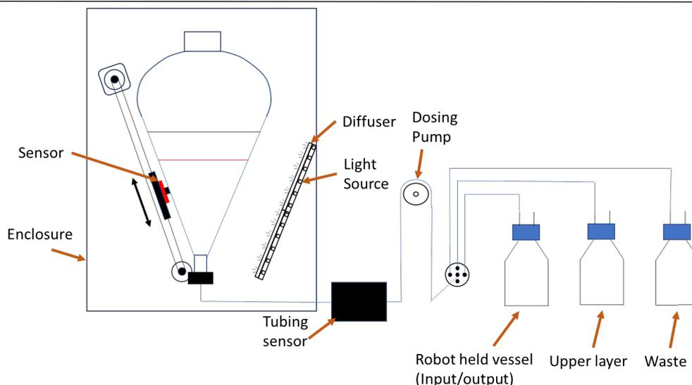
**Figure 15.** Flow diagram for LLE device. One input can be used as input output for the robot arm to load the device.
