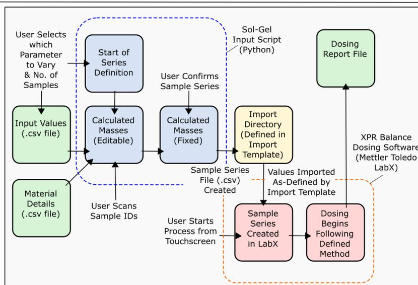
**Figure 9.** The flowchart shows the use of the input application to define a sample series for dosing and begin the dosing process. The input application runs on the instrument PC connected to the balance. The form of files used for 'Input Values' is shown in Figure 8.
