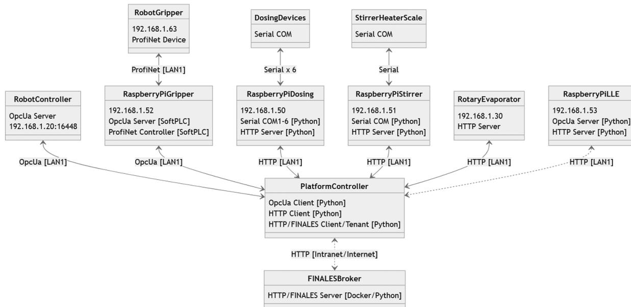
**Figure 18.** Communication architecture of the robotic platform at Fraunhofer ISC displays hard- and software components and communication protocols in between.
