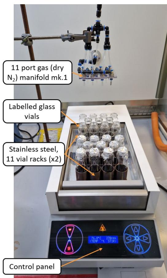
**Figure 5.** Heavy duty RS9000 heater/shaker (Electrotherm) reaction stage containing two racks of 11 samples each. The prototype gas inlet manifold, allowing the flow of dry N<sub>2</sub> into the reaction vials during shaking, is also pictured.
