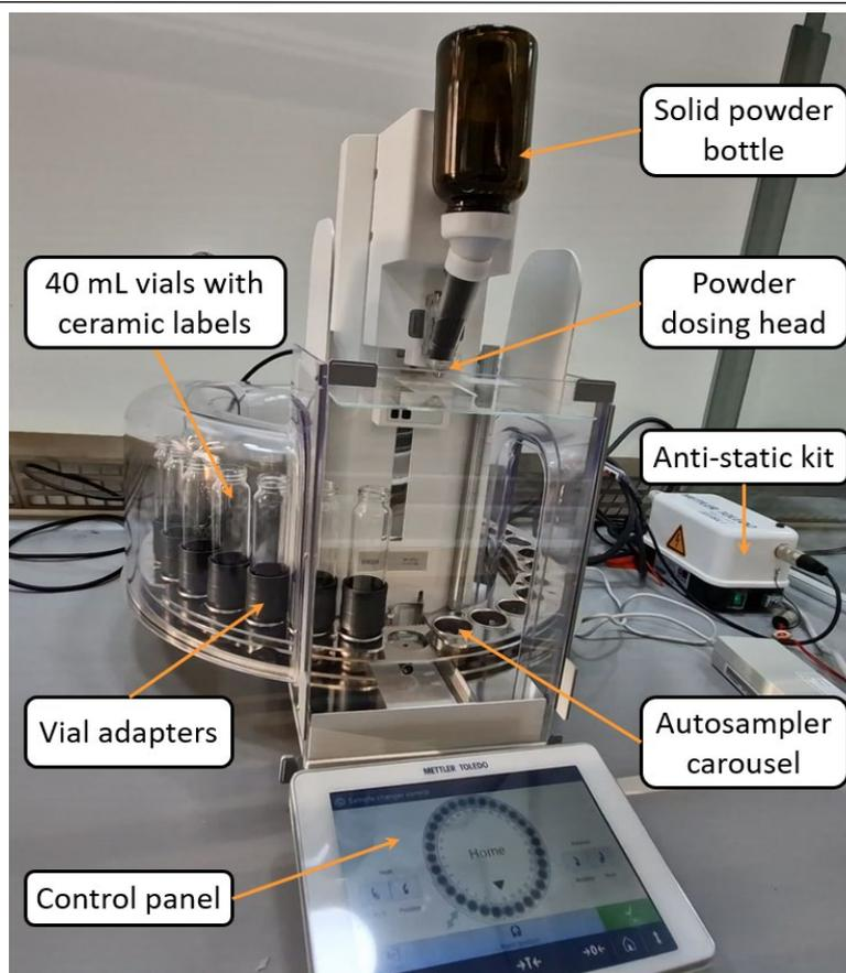
**Figure 2.** The XPR204 automated balance and sample carousel in place in the fumehood, with the NMC622 designated dosing head and bottle in place.
