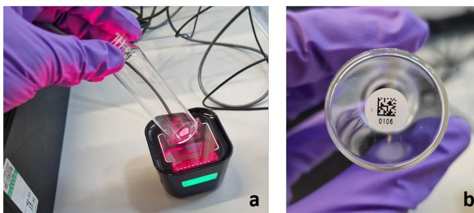
**Figure 4.** (a) USB PoS barcode reader attachment to the instrument PC running the LabX software and (b) the ceramic 2D array label, 10-digit code with human readable 4-digit code, on the base of the glass sample vial.
