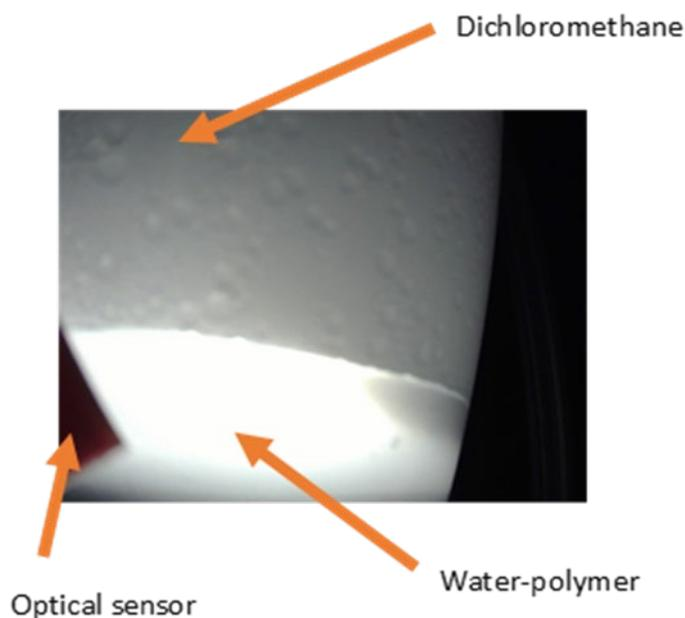
**Figure 20.** Image of the interface between the solvent dichloromethane (upper foamy layer) and the water-polymer solution (lower transparent layer) as the optical sensor camera crosses in front of it during a scan of the settling process.
