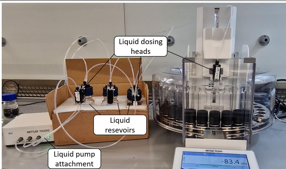
**Figure 3.** The XPR204 automated balance and sample carousel with the liquid dosing pump connected to the liquid reservoirs and dedicated liquid dosing heads.
