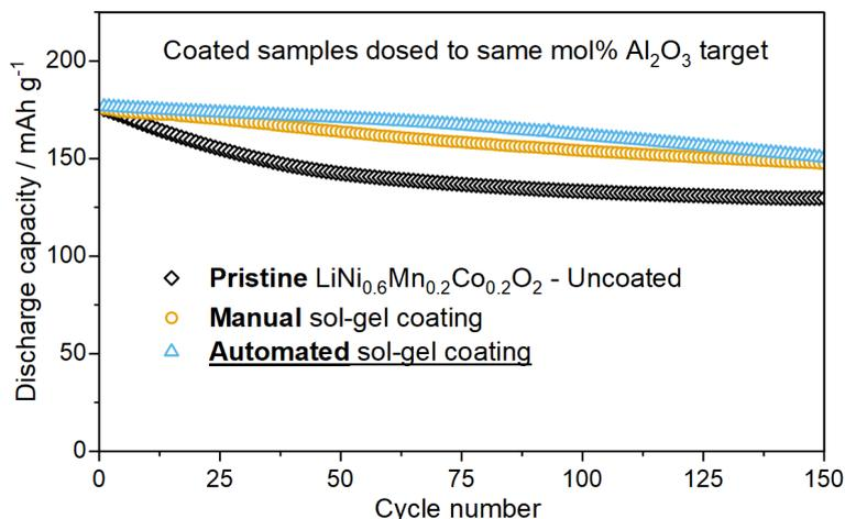
**Figure 13.** Electrochemical performance of Li|NMC622 half cells prepared using uncoated NMC622 material and the NMC622 with an Al<sub>2</sub>O<sub>3</sub> coating prepared by the manual and automated procedures.
