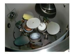
Figure 13: Possible design of the future magnetron sputtering apparatus connected to a glove box (expected 10/2021). View of a group of 3 targets in confocal geometry, similar to the one that will be used to generate the combinatorial films
