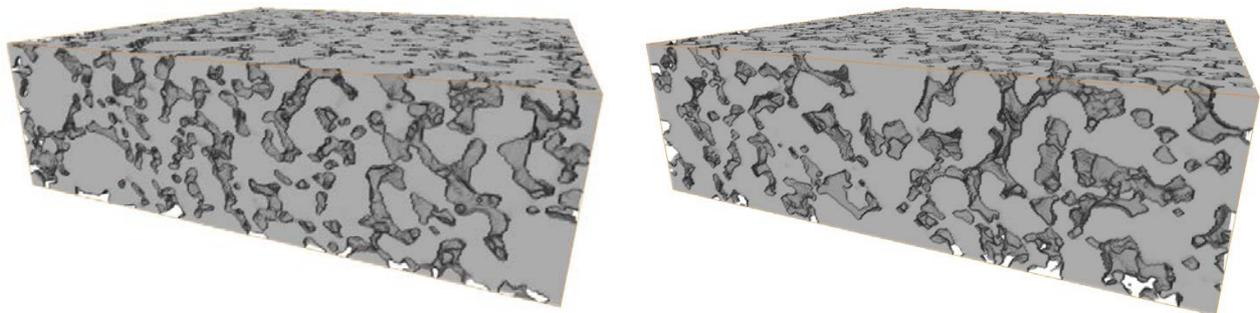
**Figure 11. Example of electrode structure data, showing 3D visualizations of (left) a cutout from tomographic image data and (right) a stochastic model realization of a Li-ion battery negative electrode. Reproduced with permission from Ref. [9].**
