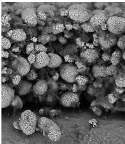
**Figure 6. Cross-section image of a Li-ion composite positive electrode showing the active material particles held together with a polymer binder cast on a foil current collector.**
