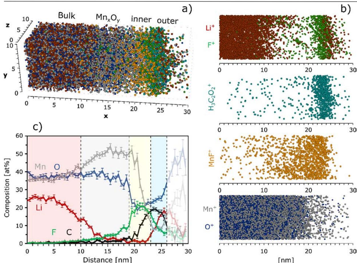
**Figure 8. Atomic resolution analysis of the cathode electrolyte interface on LMO. a) 3D APT ion map of a sub-volume ( $30 \times 10 \times 10 \text{ nm}^3$ ) of the LMO tip and b) 2D projections, normal to the  $xy$  plane, of the single ion maps c) Composition profiles of the atomic fractions for Li, Mn, O, F and C. Reproduced with permission from Ref. [7].**
