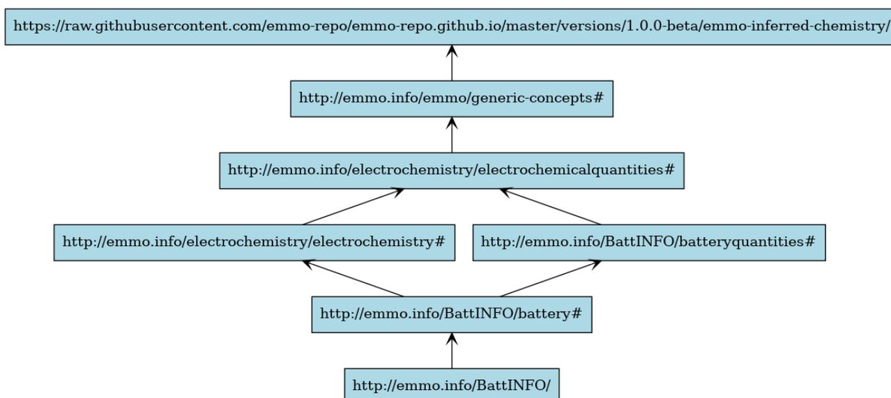
Figure 2. Overview of the BattINFO import structure.
